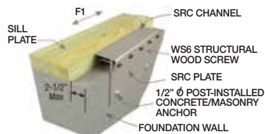
Mitek SRC requires PowerStud® anchors TYPICAL SRC INSTALLATION ON RECTANGULAR FOUNDATION
